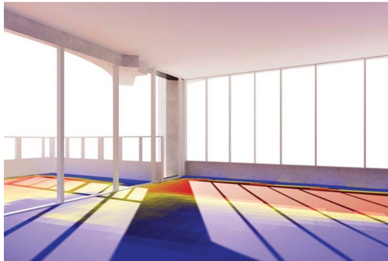
IMAGE OF SOLAR COVERAGE ON WESTERN TERRACE
